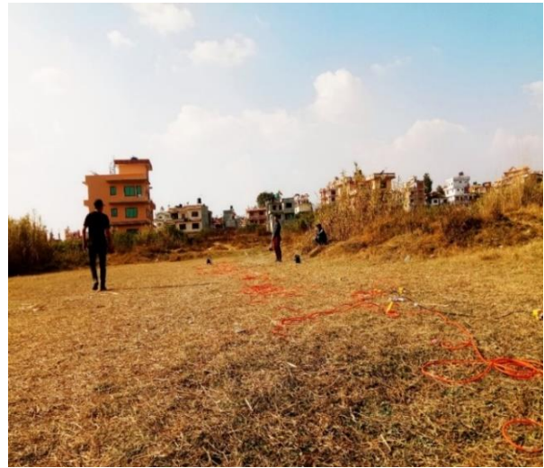
Fig2: Seismic field survey (MASW) performed behind the Kathmandu Medical College, Duwakot, Ward 2, Changunarayan Municipality
