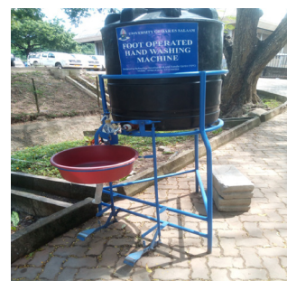
Figure 1: Single-Tap foot-operated handwashing machine.
