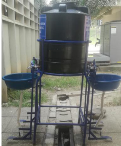
Figure 3: Double-tap Foot-operated Handwashing Machine.
