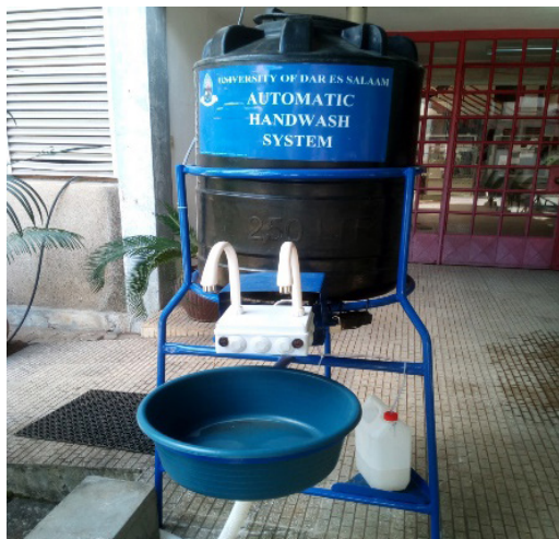
Figure 6: Automatic Handwashing Machine on site.
